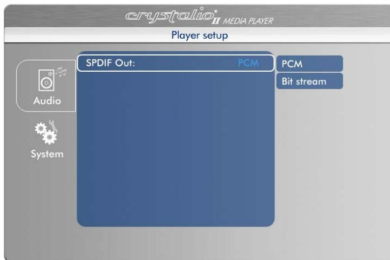
SPDIF (Sony/Philips Digital Interface Format) is a protocol to govern the data transferred using the Digital Audio Outputs of *Crystalio II*.
